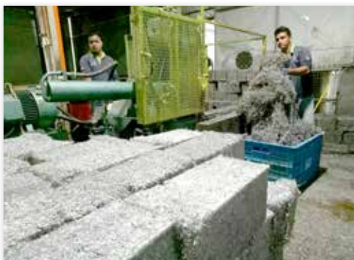
Scrap metal components such as steel, aluminum and titanium are compacted at our factory site before they are disposed to a licensed local scrap metal recycler.
